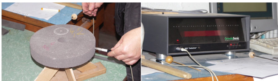
Measurement using Grindo Sonic MK 5 “Industrial”, Belgium
