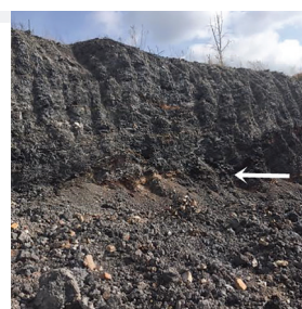
Stratification of air-cooled blast-furnace slag at the Kladno deposit and comparison of the FTIR spectra of the slag and its alkali-activated form
