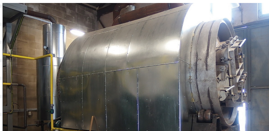
Rotary kiln for the large-scale processing of polyethylene waste
