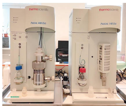
PASCAL 140 + PASCAL 440 EVO mercury porosimeters, Thermo Scientific
